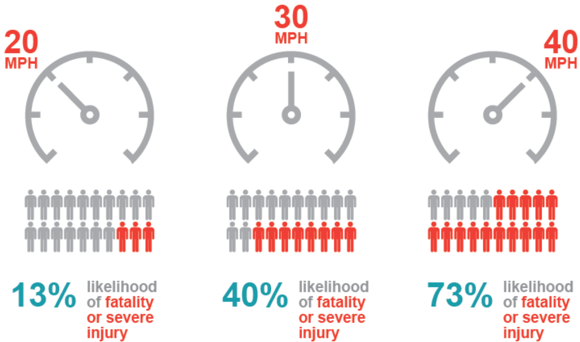
Figure 2: Relation Between Motorist Speeds and Rate of Pedestrian Fatality or Severe Injury
